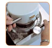
Once the heating time has elapsed, flip the pressure chamber or plate carrier over the model and seal.
