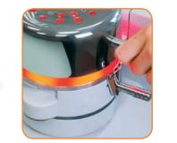
After preheating for approx. 1 minute, swivel the heater over the material.
