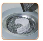
Place model on the platform or embed it into the pellets.
