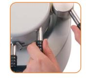
After heating time has elapsed, swivel pressure chamber over the model and close locking handle.
